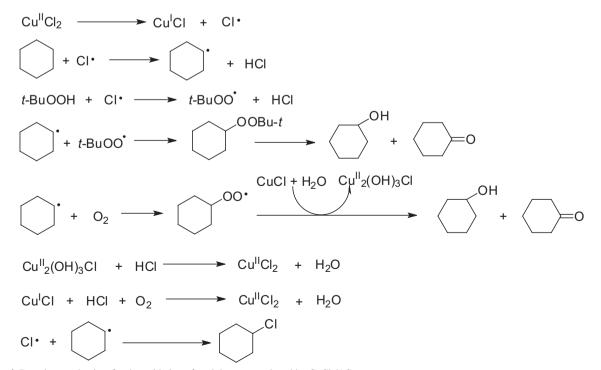
Figure 4. Reaction mechanism for the oxidation of cyclohexane catalyzed by CuCl<sub>2</sub>/AC.
