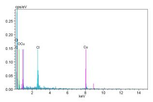
Figure 3. Energy dispersive X-ray spectrum of supported CuCl<sub>2</sub>.
