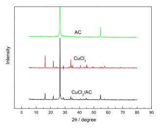
Figure 2. XRD of AC, CuCl<sub>2</sub> and CuCl<sub>2</sub>/AC.
