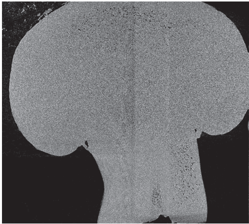
Figure 1. Interior microtomography ( \mu -CT) of the precooked mushroom (SkyScan 1173, 1 pixel = 12.5 \mu m).
