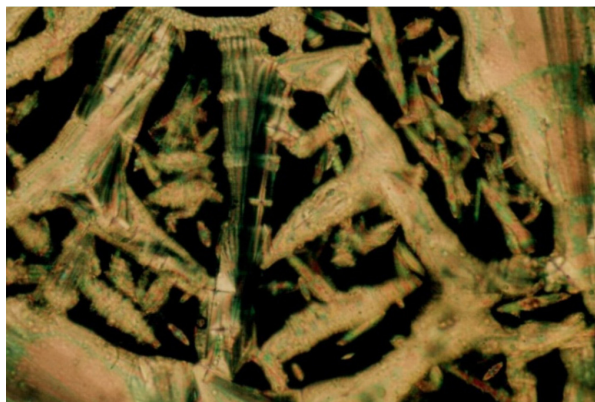
Figure 2. Growth of SmA bâtonnets (bright) of fan focal-conic texture of SmA mesophase upon cooling at 161 °C of thiazoline 6i .
