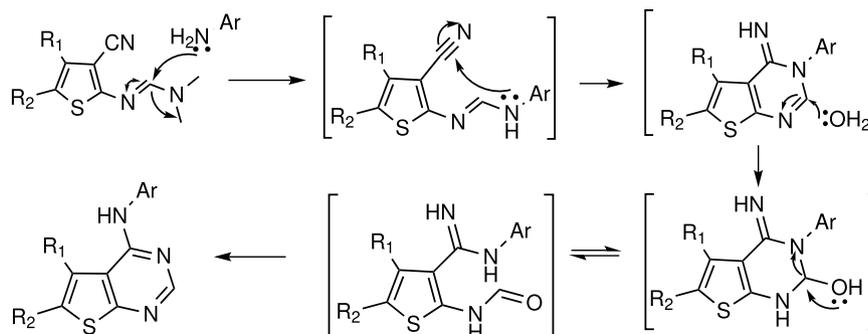
**Scheme 2.** Proposed mechanism for the Dimroth rearrangement.
