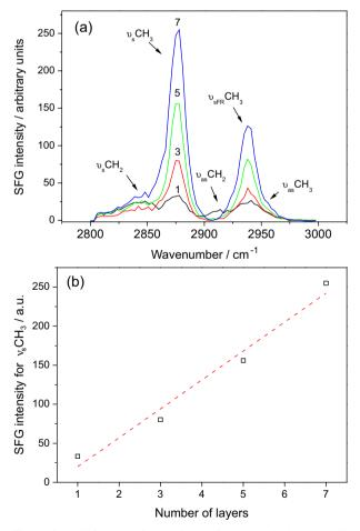
**Figure 6.** (a) SFG spectra for the glass surface covered with several Zn stearate layers (the attributions of the correspondent stretching modes are indicated according to Table 2); (b) intensity of the peak associated with the symmetric stretching of  $CH_3$  as a function of the number of layers.
