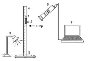
**Figure 1.** Scheme of the experimental apparatus used to generate the drops and image acquisition: (1) fluid reservoir tube (burette); (2) valve to release drop; (3) lighting system; (4) ruler; (5) impact base; (6) camera and (7) computer.
