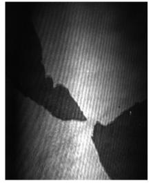
**Figure 4.** BAM image of a 3-layer LB film of zinc stearate on glass, before drop impact. The image size is 300 (H)  $\times$  375 (V)  $\mu$ m<sup>2</sup>. Brighter regions correspond to thicker films. The nearly vertical pattern of fine lines is an artifact due to interference of the laser reflection on the back side of the substrate.
