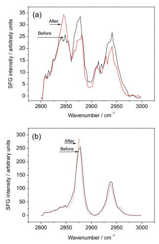
**Figure 7.** SFG spectra for the surfaces covered with (a) one and (b) seven layers, before and after the impact of three droplets.
