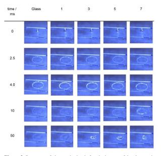
**Figure 2.** Sequence of photos obtained after the impact of droplets against glass surface and on glass surface covered with 1, 3, 5, and 7 monolayers. At the left are indicated the times (in ms) after the first contact of the drop with the surface in which the photos were taken.
