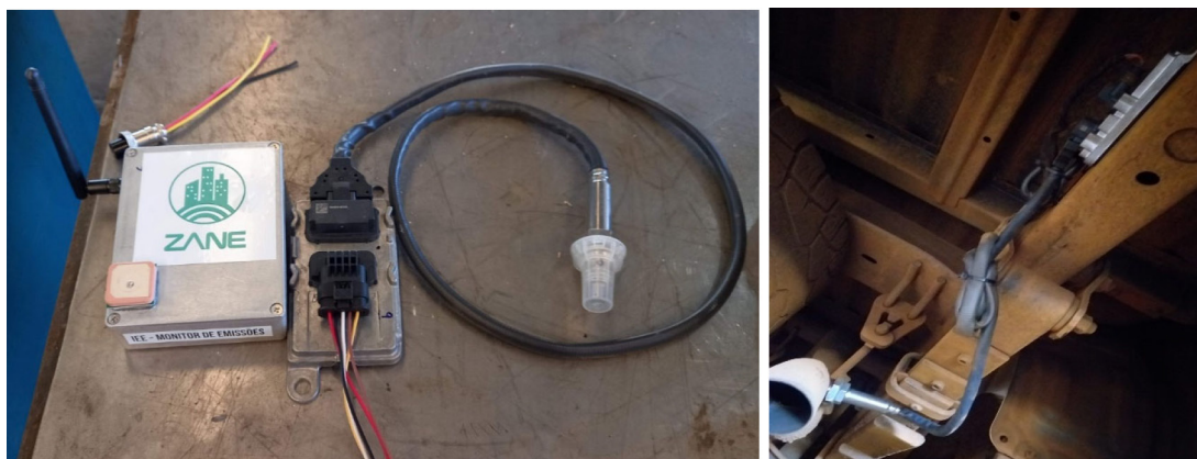
Figure 1. NO x sensor and control module installed in the vehicles tested for this study.
