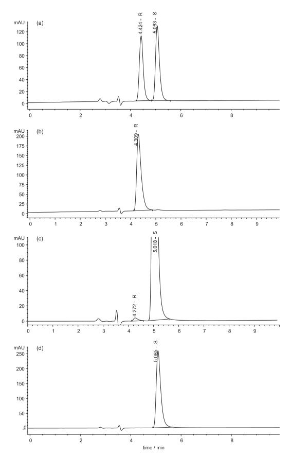
**Figure 2.** (a) Enantiomeric resolution of repaglinide; (b) HPLC chromatogram of (R)-repaglinide; (c) HPLC chromatogram of (S)-repaglinide bulk sample (0.5 mg mL<sup>-1</sup>) spiked with (R)-enantiomer (0.5%); (d) HPLC chromatogram of (S)-repaglinide tablet.
