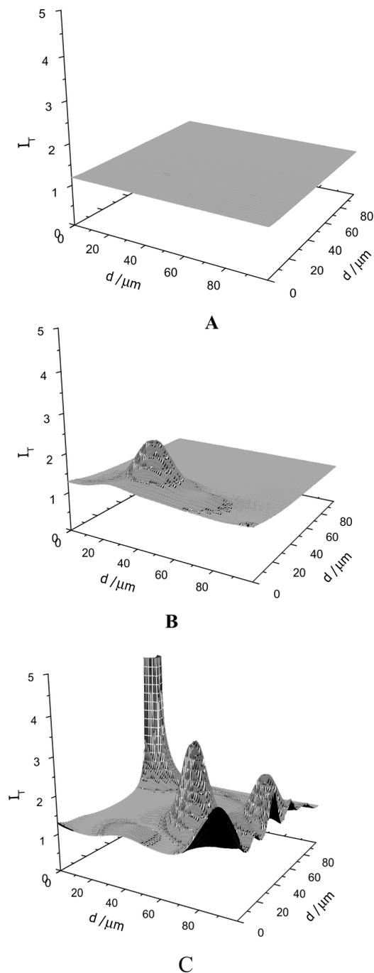
**Figure 8.** SECM surface-plot images of GCE (A), MWCNT modified electrode (B) and MWCNTsox modified electrode (C). Concentration of dispersion: 1 mg mL<sup>-1</sup>, 1 mmol L<sup>-1</sup> FeOH in 0.2 mol L<sup>-1</sup> phosphate buffer (pH 7.4) was used as a redox mediator.
