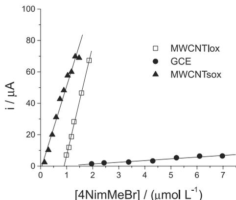
**Figure 9.** Calibration curves of 4-NimMeBr obtained at bare GCE ( $i_p$ :  $-0.77 + 0.01[4\text{-NimMeBr}]$ ) at modified with both large (CNTlox) ( $i_p$ :  $-62.86 + 6.97[4\text{-NimMeBr}]$ ) and short (CNTsox) ( $i_p$ :  $-2.52 + 5.34[4\text{-NimMeBr}]$ ) oxidized MWCNT. MWCNT:  $4 \text{ mg mL}^{-1}$   $0.1 \text{ mol L}^{-1}$  Britton-Robinson buffer, pH 2. Scan rate:  $100 \text{ mV s}^{-1}$ . Curves were obtained using LSV (bare GCE) or ASV (Modified GCE) techniques.
