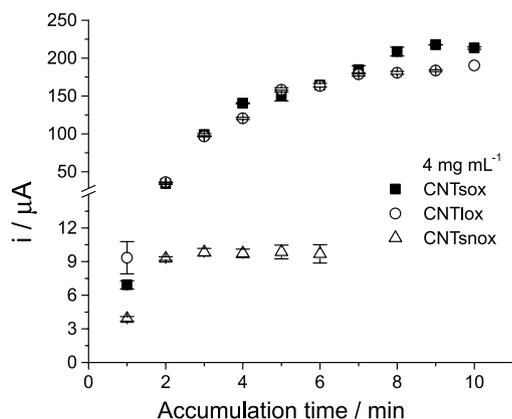
**Figure 7.** Dependence of the peak current with the accumulation time on GCE modified with different MWCNT: MWCNT short and oxidized = CNTsox; MWCNT large and oxidized = CNTlox; MWCNT short and non-oxidized = CNTsnox. [4-NimMeBr]:  $3 \times 10^{-6}$  mol L<sup>-1</sup>. MWCNT: 4 mg mL<sup>-1</sup>, 0.1 mol L<sup>-1</sup> Britton-Robinson buffer, pH 2. (Obtained with LSV, scan rate 100 mV s<sup>-1</sup>).
