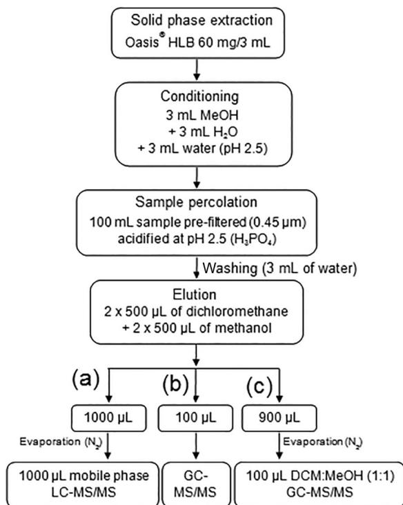
**Figure 4.** Schematic representation of the solid phase extraction (SPE) approach applied for pesticide multiresidue determination in water by LC-MS/MS in (a) and GC-MS/MS in (b). The procedure (c) was used for determination of aldrin, dieldrin and chlordane.
