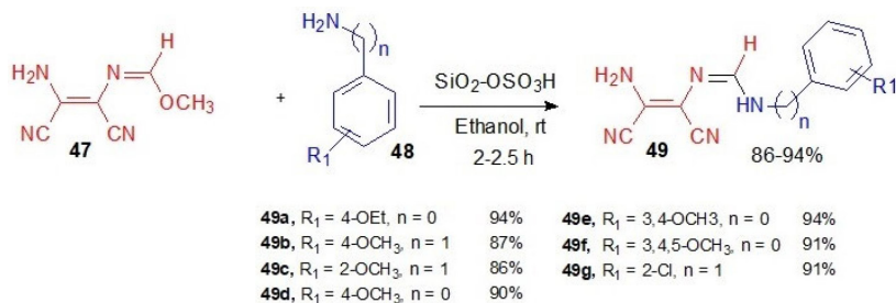
Scheme 15. Synthesis of amidines from amines and imidoesters catalyzed by acidified silica. 84
