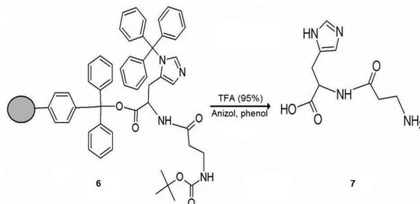
**Scheme 4.** Deprotection of *tert*-butyloxycarbonyl (Boc) group and cleavage from the resin. TFA: Trifluoroacetic acid.
