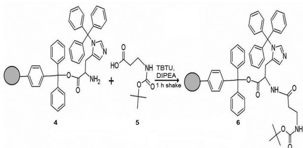
**Scheme 3.** Coupling of second amino acid Boc- $\beta$ -alanine-OH to the resin. DIPEA: *N,N*-Diisopropylethylamine; TBTU: *O*-(benzotriazol-1-yl)-*N,N,N',N'*-tetramethyluronium tetrafluoroborate.
