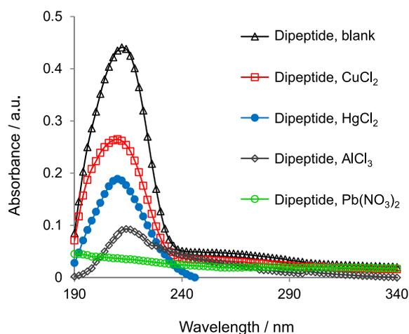
**Figure 3.** Ultraviolet visible (UV-Vis) absorption spectra of dipeptide ( $10^{-4}$  mol L $^{-1}$ ) with  $AlCl_3$ ,  $CuCl_2$ ,  $HgCl_2$  and  $Pb(NO_3)_2$ .
