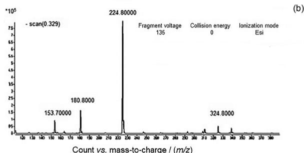
**Figure 2.** Liquid chromatograph-mass spectrometry (LC-MS) chromatogram of dipeptide (histidine- $\beta$ -alanine): (a) +scan; and (b) -scan.
