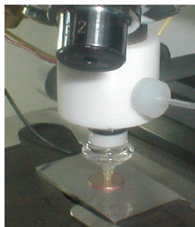
Figure 1. Overview of the experimental set-up with electrochemical microcell (adapted from reference 33).
