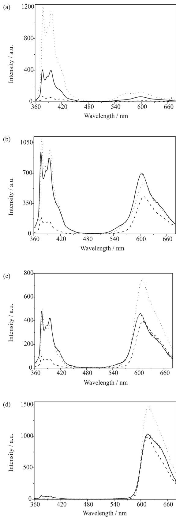
**Figure 6.** Steady-state fluorescence spectra ( $\lambda_{exc} = 348$  nm) of spin coated MEH-PPV blends with PS-*py* (—), SEHAMA-*py*-9 (---) and SEHAMA-*py*-19 (.....) containing: (a) 0.1, (b) 0.5, (c) 1.0 and (d) 5.0 wt%.
