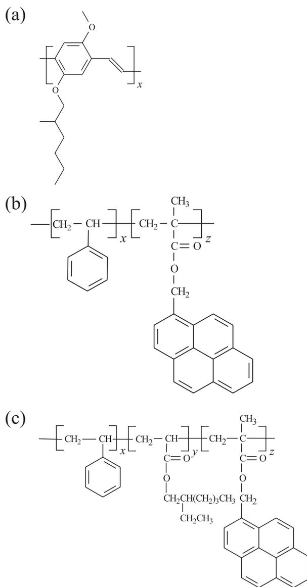
**Figure 1.** Chemical structures of the conjugated polymers (a) MEH-PPV, (b) poly(styrene-*co*-1-methylpyrenyl methacrylate) (PS-*py*) and (c) poly(styrene-*co*-2-ethylhexyl acrylate-*co*-1-methylpyrenyl methacrylate) (SEHAMA-*py*).
