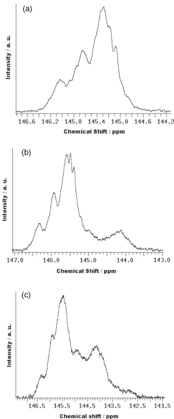
**Figure 2.**  $^{13}\text{C}$  NMR spectra in  $\text{CDCl}_3$  in the region of the  $\text{C}_\alpha$ -methynic units of the styryl units for the copolymers (a) PS-*py*; (b) SEHAMA-*py*-9; (c) SEHAMA-*py*-19.
