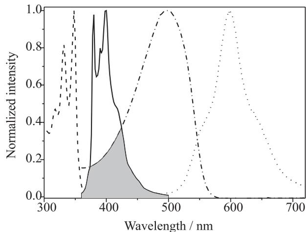
**Figure 4.** Normalized electronic absorption and fluorescence spectra of spin coated polymer films: pyrenyl moieties of SEHAMA-*py*-9 copolymer absorption (---) and emission (—) ( $\lambda_{exc} = 348$  nm); blend of MEH-PPV (0.1 wt%) and polystyrene - absorption (-·-·-) and emission (····) ( $\lambda_{exc} = 460$  nm). The filled area represents the spectral overlap between pyrenyl group emission (donor) spectrum and the MEH-PPV absorption spectrum (acceptor).
