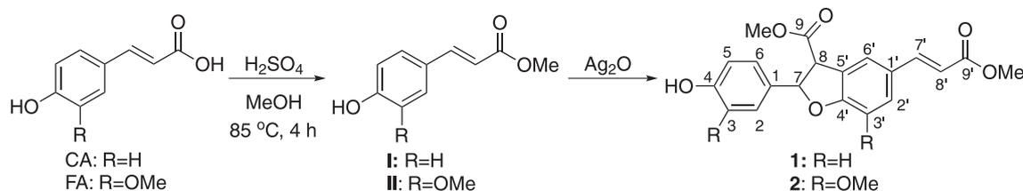
**Scheme 2.** Synthesis of the dihydrobenzofuran neolignans **1** and **2** by silver(I)-oxide oxidative coupling of methyl *p*-coumarate (**I**) and methyl ferulate (**II**), respectively (adapted from references 4,7,11,16).
