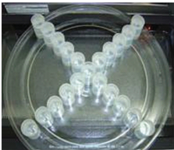
Figure S2. Experimental set up for evaluation of the distribution of microwave radiation within the microwave oven cavity.
