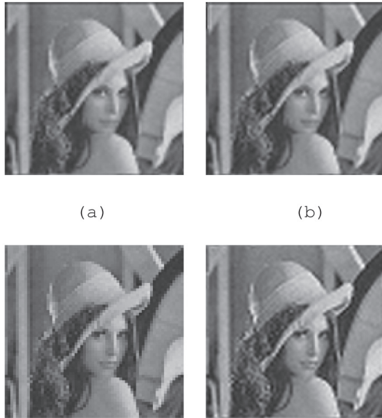
Figure 5: Interpolation Results of Lenna Image: (a) Bicubic. MSE=339, a_e=0.56 . CPU=0.7 s. (b) Cubic Spline. MSE= 342, a_e=0.57 . CPU=1.1 s. (c) Iterative Regularized (100 iterations). MSE= 313, a_e=0.66 . CPU=8.6 s. (d) Inverse Regularized. MSE=223, a_e=0.78 . CPU= 17.2 s.
