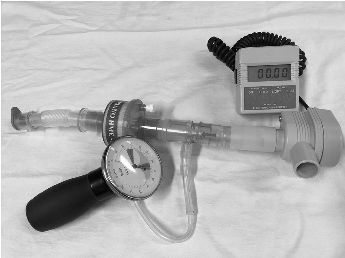
**Figure 2.** Experimental setup used for voluntary breath stacking. The monitoring system, based on inspiratory capacity (measured with a respirometer), was coupled to a one-way valve connected to an analog manometer. A bacterial filter was used for patient coupling. For involuntary breath stacking, a resuscitator bag was connected to the respirometer outlet.
