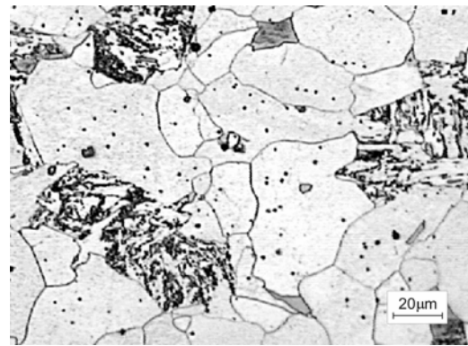
Figure 3. Optical microscopy of the CMnMo weld metal after the normalizing heat treatment showing equiaxed ferrite grains and ferrite-carbide aggregate.
