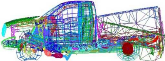
Figure 2. Chassis eigenmode of a pickup at f=11.2\text{ Hz} .
