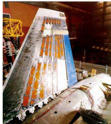
Figure 1. An example of direct-active system: F-18 Fighter instrumented fin with piezoelectric actuators for buffeting control. From Nitzsche et al. (2001).
