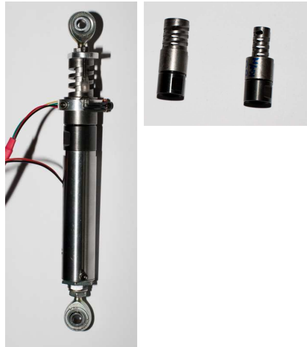
Figure 5. Active or Adaptive Pitch Link (APL) device (left). Secondary-path spring components, of 163 kN/m and 256 kN/m (right).
