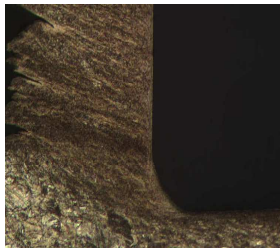
Figure 4. Photomicrograph of samples at 100 x magnification ( \text{CuZn30} , \gamma = 0^\circ , r = 100 \mu\text{m} , V_c = 0.75 \text{ m/min} , t = 50 \mu\text{m} ).
