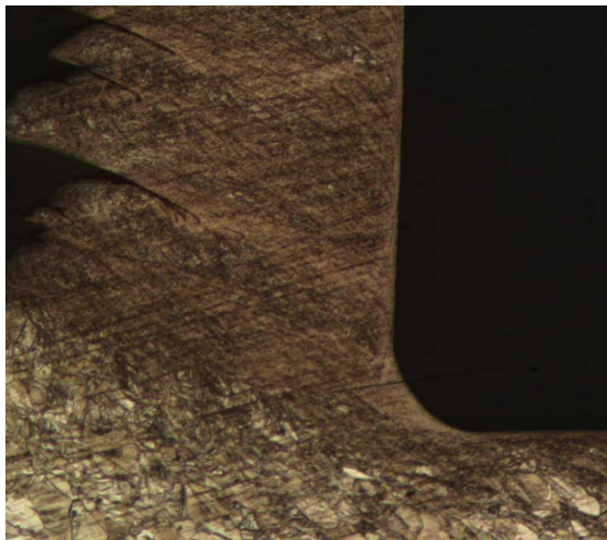
Figure 6. Photomicrograph of samples at 100 x magnification (CuZn30, \gamma = 0^\circ , r = 100 \mu\text{m} , V_c = 0.75 \text{ m/min} , t = 150 \mu\text{m} ).
