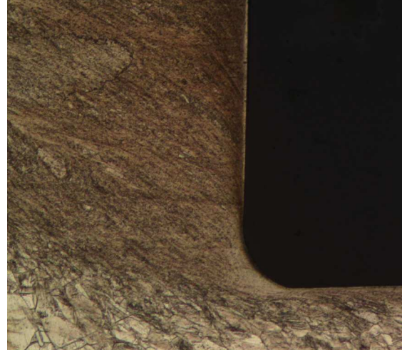
Figure 7. Photomicrograph of samples at 100 x magnification (CuZn30, \gamma = 0^\circ , r = 150 \mu\text{m} , V_c = 0.5 \text{ m/min} , t = 150 \mu\text{m} ).
