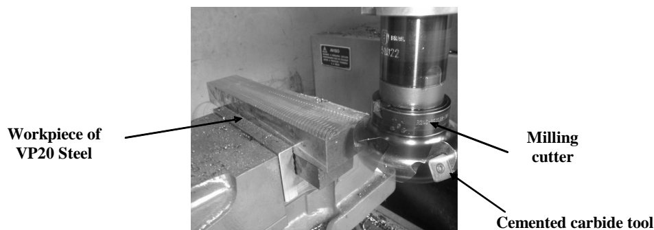
Figure 5. Set-up of the workpiece and the milling cutter.
