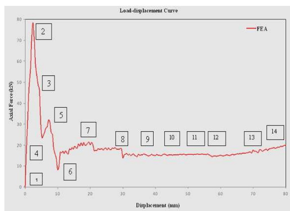
Figure 11. Load-displacement diagram from FEA model.
