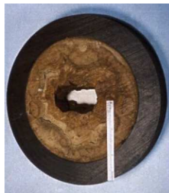
Figure 1. Wax deposition blockage in pipelines; adopted from Fogler (2004).
