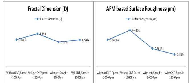
Figure 19. Fractal dimension and surface roughness analysis for different machining conditions.
