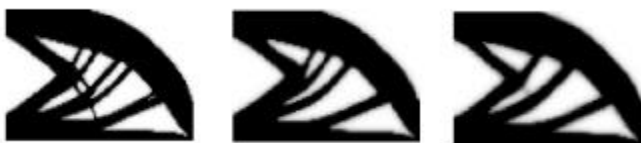
Figure 6. Results obtained for three different filter radiuses. The radius is increased from left to right.
