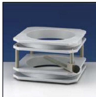
Fig. 2 - Helmholtz coil from Brockhaus Messtechnik used in the tests.
