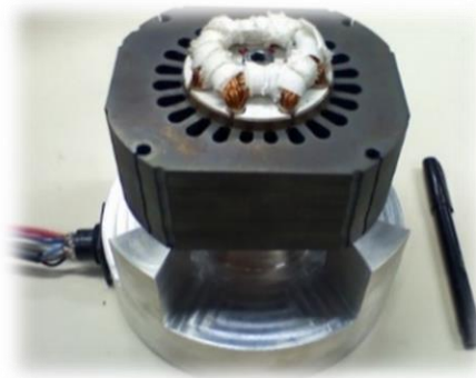
Fig. 5. Magnetic head used for exciting the unwound stator sample.
