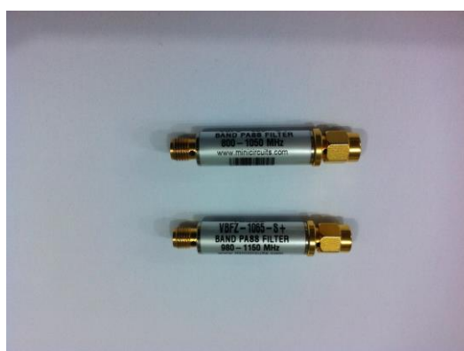
Fig. 6. 925MHz and 1065MHz filters used for testing.
