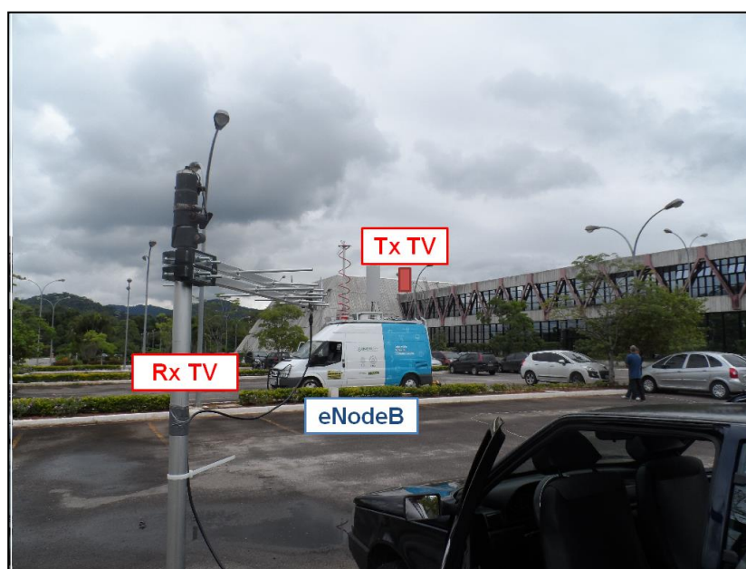
Fig. 4. Ground view of the measurement setup of LTE interference on digital TV
