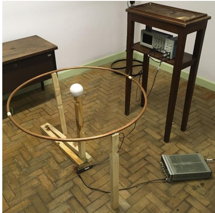
Fig. 9. Test setup with Kanda Antenna and a small current loop (as the DUT)
