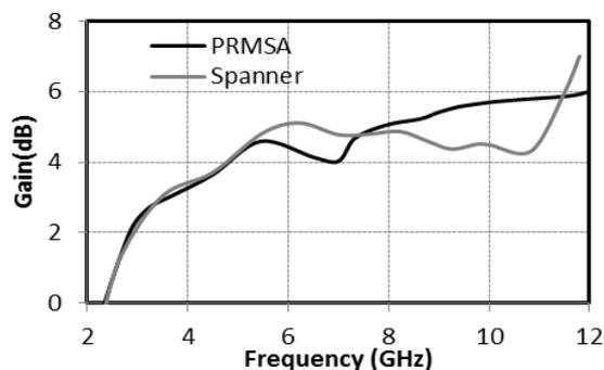
Fig. 10. Simulated gain Vs. frequency of proposed antenna
