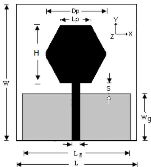
Fig.1. A regular hexagonal shape monopole antenna
