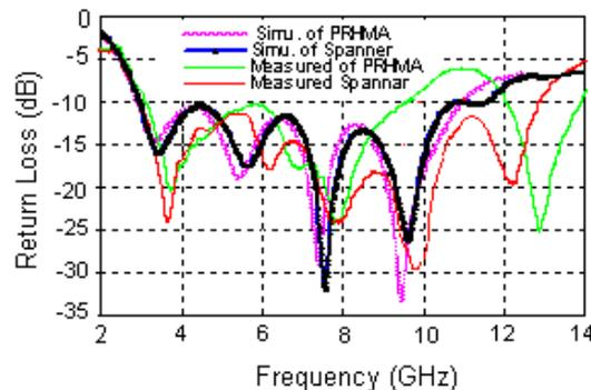
Fig.7. Comparison of the return loss characteristics (simulation and measured) of PRHMA and spanner shape monopole antenna
