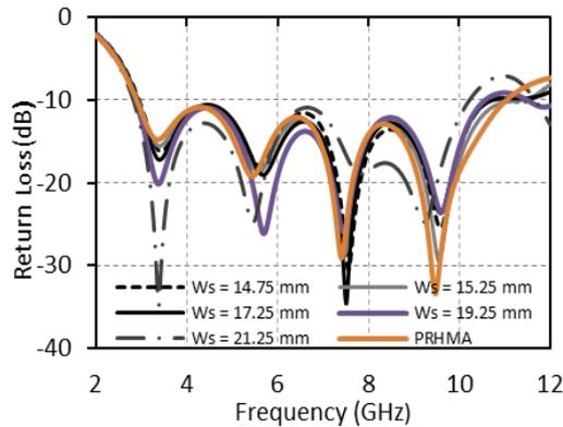
Fig.5. Simulated return loss characteristics for various lengths of  $W_s$
