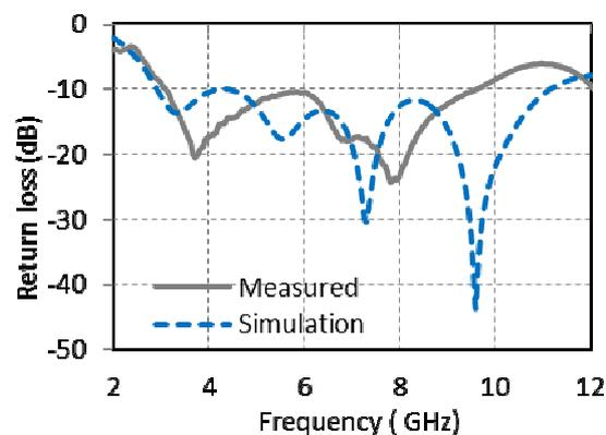
Fig.4 Return loss characteristics of Fig. 1
