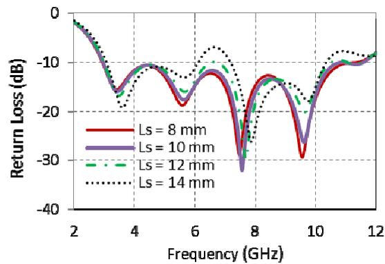
Fig.6. Simulated return loss characteristics for various widths of  $L_s$
