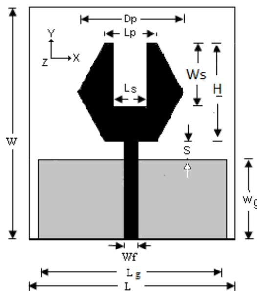
Fig.2. A defected regular hexagonal shape (spanner shape) monopole antenna
