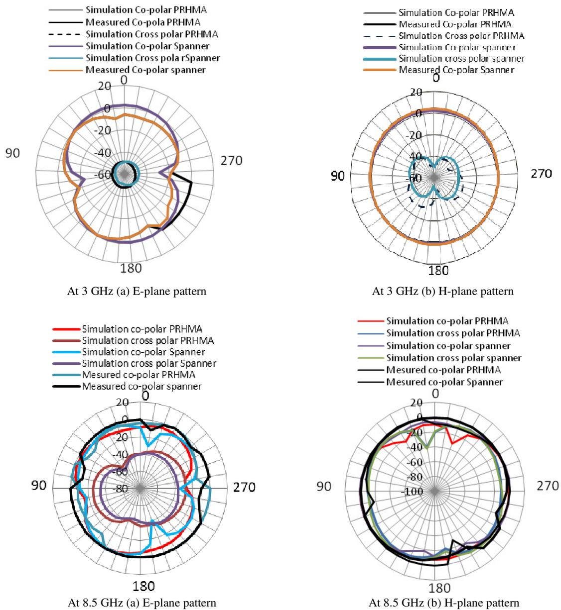
Fig.8. Simulation and measured E-plane and H- plane radiation pattern (Fig. 2 and Fig. 3)
