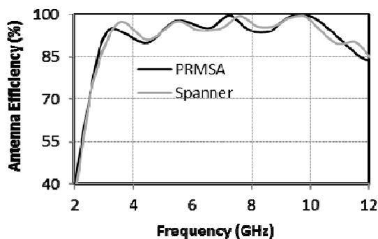
Fig. 9. Simulated antenna efficiency Vs. frequency of proposed antenna
