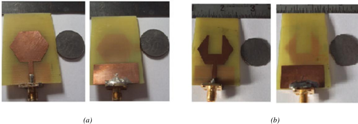
Fig. 3. Fabricated antennas (a) prototype PRHMA (b) spanner antenna; Top plane (left side), bottom plane (right side)
