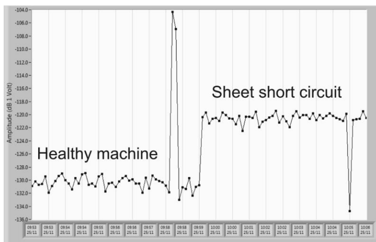
Fig. 25. Evolution of the 862.5 Hz component amplitude as a function of measurements along the time.
