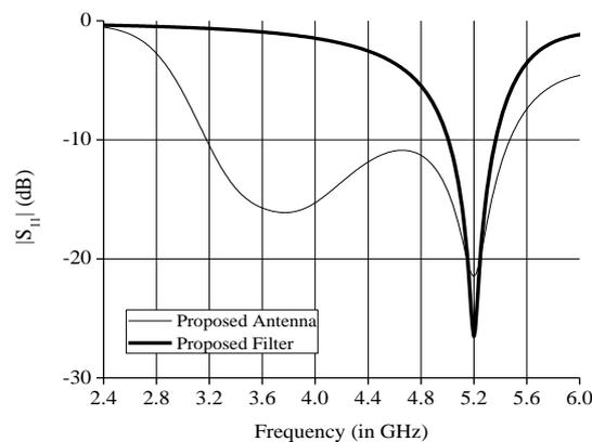
Fig. 5. Return loss curves for proposed antenna and filter.
