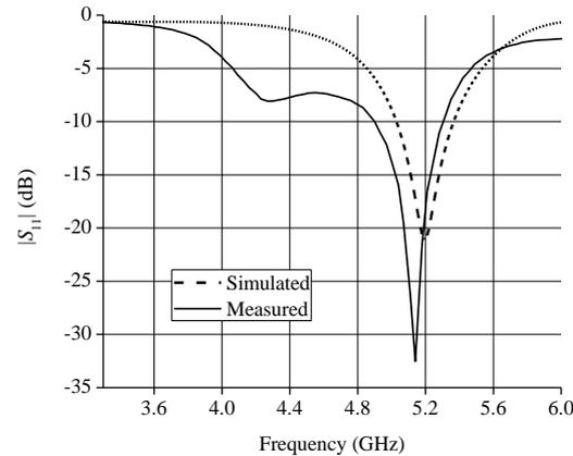
Fig. 8. Simulated and Measured return loss curve
