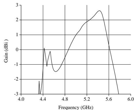
Fig. 9. (b) Simulated Gain curve
