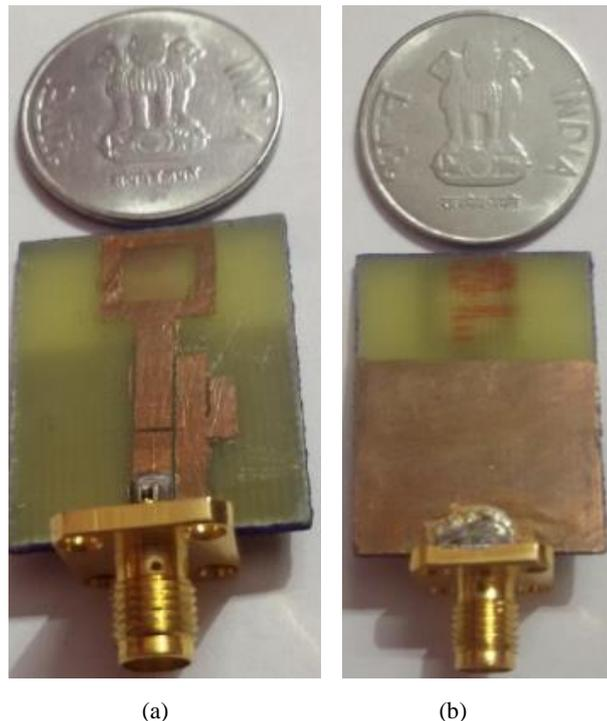
Fig. 7. Photograph of the prototype filtenna (a) Top view and (b) Bottom view.
