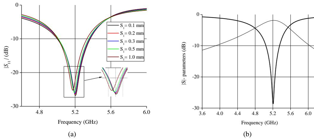
Fig. 4. (a) Simulated return loss for different gap spacing (b) Filter response at  $S_1 = 0.2$  mm.
