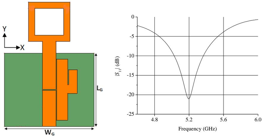
Fig. 6. (a) Structure of Proposed Filtenna; (b) Simulated return loss response.
