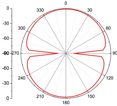
Fig. 10. (a) E-plane radiation pattern
