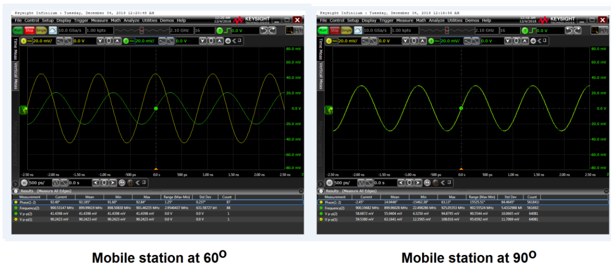
Fig. 10. Oscilloscope screen views of received signals from Antenna 1 and Antenna 2 at the same time.
