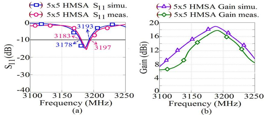
Fig. 14. (a)  $S_{11}$  plots for  $5 \times 5$  HMSA array with  $\lambda_g$  spacing and its (b) gain plots.
