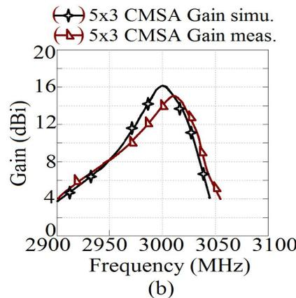
Fig. 5. (a) Planar CMSA array using  $\lambda_g$  spacing and (b) gain plots with  $\lambda_g$  spacing for  $5 \times 3$  CMSA array.
