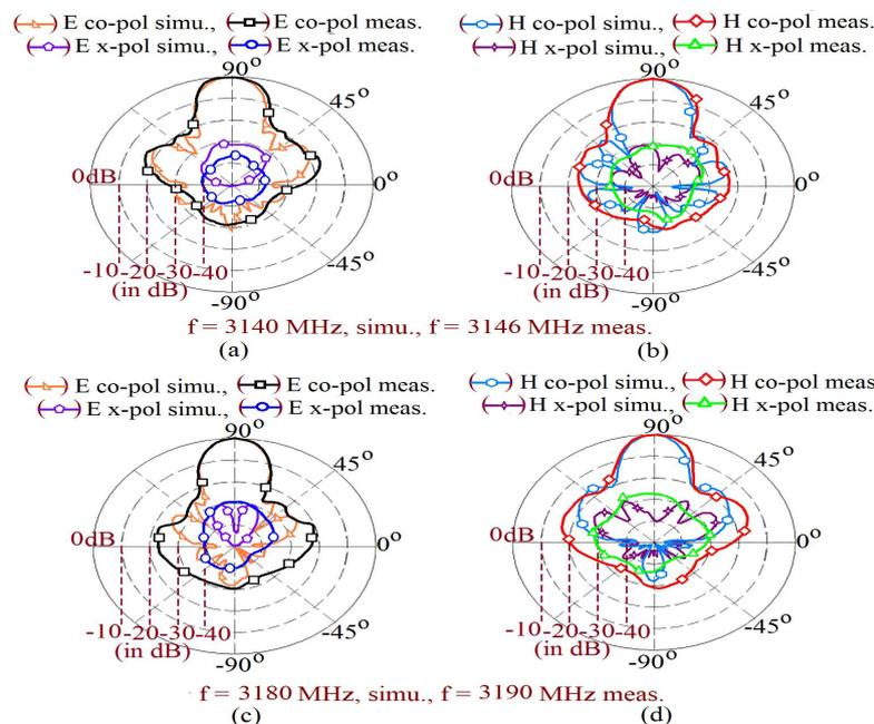
Fig. 15. (a), (b) Radiation pattern at the center frequency of the impedance BW for  $5 \times 3$  and (c), (d) for  $5 \times 5$  planar HMSA binomial array.
