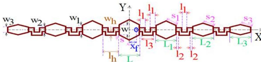
Fig. 9. Linear series fed  $7 \times 1$  binomial HMSA array.
