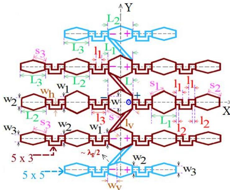
Fig. 10. Planar binomial HMSA array employed with  $\lambda_g/2$  spacing along the H-plane.
