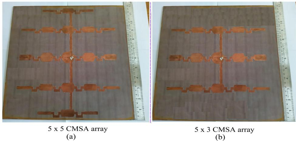
Fig. 8. Fabricated prototype of (a)  $5 \times 5$  and (b)  $5 \times 3$  CMSA arrays.
