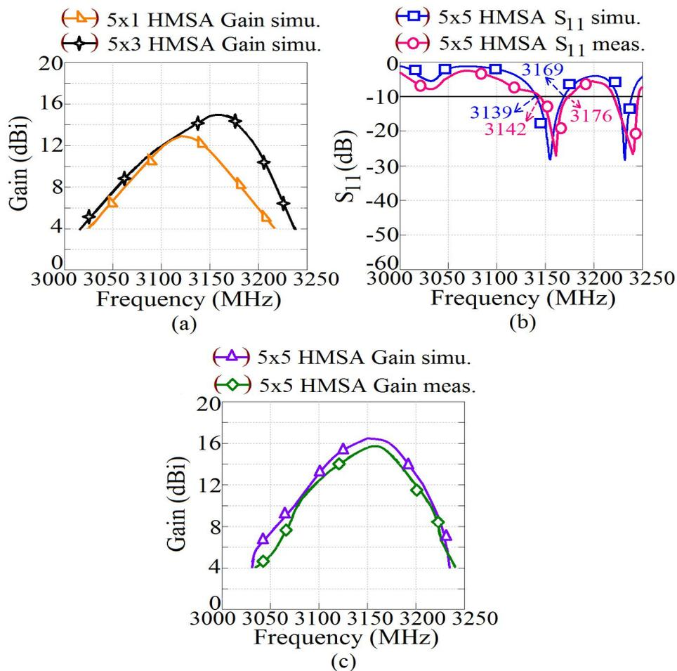
Fig. 11. (a) Gain plots for  $5 \times 1$  and  $5 \times 3$  binomial HMSA array with  $\lambda_g/2$  spacing (b), (c)  $S_{11}$  and gain plots for  $5 \times 5$  planar binomial HMSA array with  $\lambda_g/2$  spacing .
