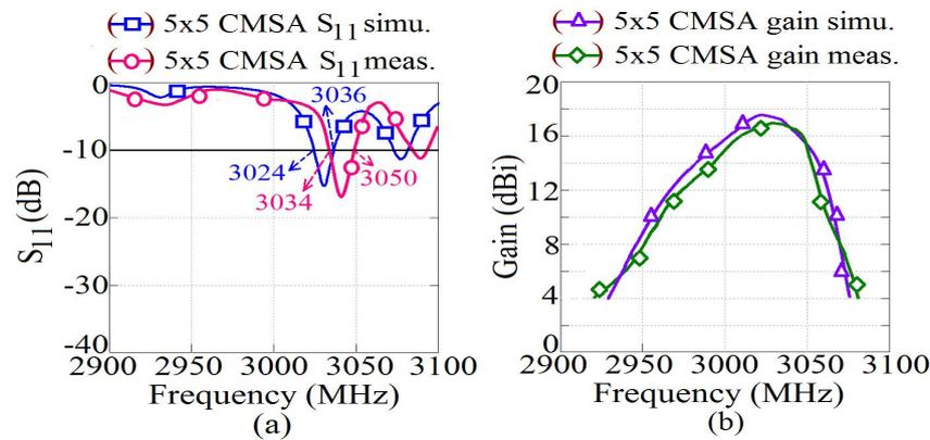
Fig. 6. (a)  $S_{11}$  with  $\lambda_g$  spacing for  $5 \times 5$  CMSA array and its (b) gain plots.
