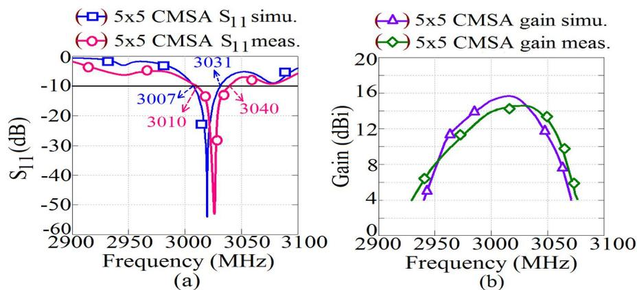
Fig. 3. (a) Reflection coefficient plots for the planar binomial CMSA array with  $\lambda_g/2$  spacing and its (b) gain plots.
