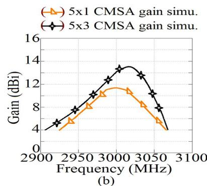
Fig. 2. (a) Planar binomial CMSA array with ' $\lambda_g/2$ ' spacing, (b) gain plots for  $5 \times 1$  and  $5 \times 3$  CMSA array.
