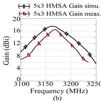
Fig. 13. (a) Planar HMSA array using  $\lambda_g$  spacing (b) gain plots with  $\lambda_g$  spacing for  $5 \times 3$  HMSA array.
