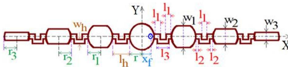
Fig. 1. Linear series fed  $7 \times 1$  binomial CMSA array (dimensions in mm).
