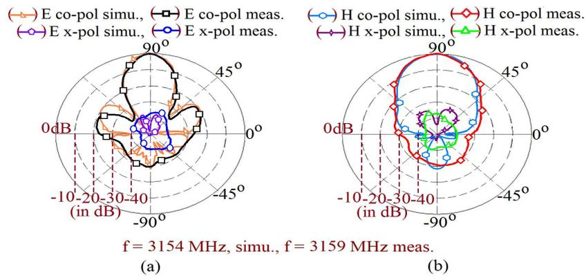
Fig. 12. (a), (b) Radiation pattern plots for  $5 \times 5$  planar binomial HMSA array with  $\lambda_g/2$  spacing.
