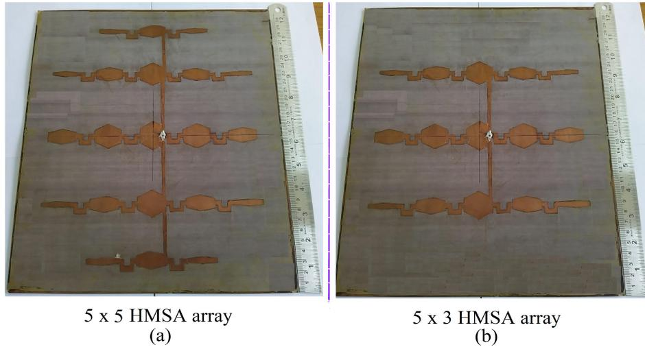
Fig. 16. Fabricated prototype of (a)  $5 \times 5$  and (b)  $5 \times 3$  HMSA arrays
