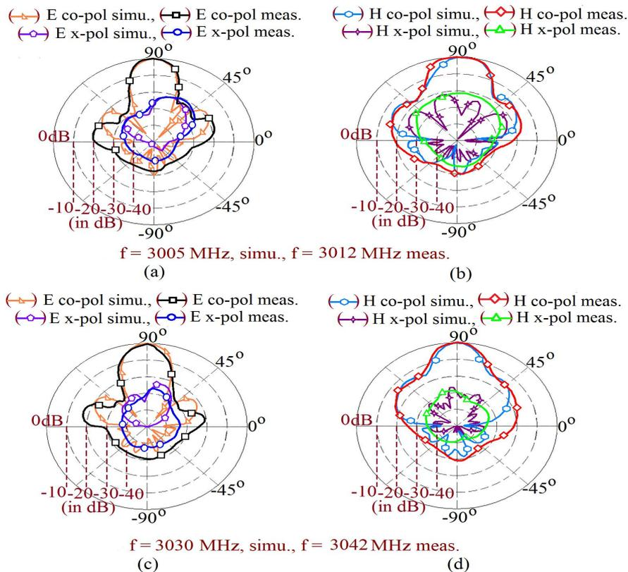
Fig. 7. (a), (b) Radiation pattern at the center frequency of BW for  $5 \times 3$  and (c), (d) for  $5 \times 5$  CMSA arrays.
