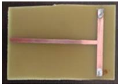
Fig. 2. T- resonator built in FR4 material.
