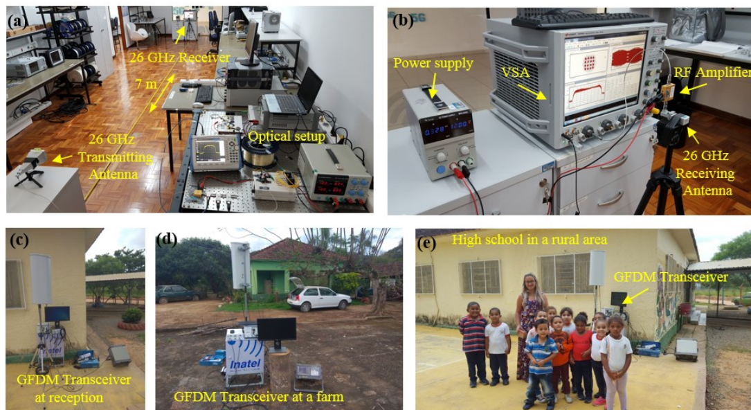
Fig. 6. Photographs of the OWN implementation: (a) Indoor environment; (b) Zoom-in view of the indoor receiver side; (c) and (e) GFDM transceiver at a high school in a rural area; (d) GFDM at a farm.
