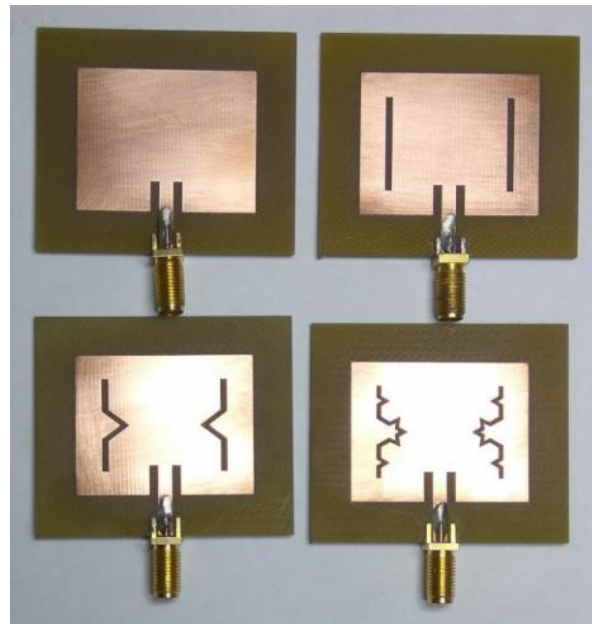
Fig. 6. Evolution of the iteration in the patch antennas.
