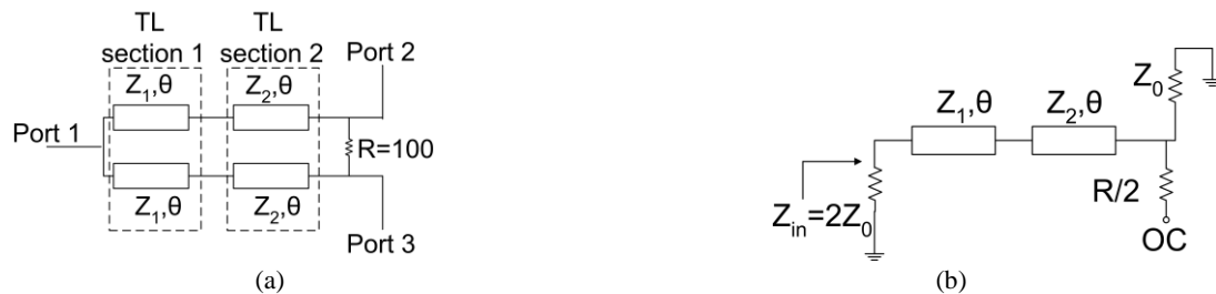
Fig. 1. WPD with two TL sections (a) structure proposed in [3] and (b) bisected (half) circuit for even mode analysis.
