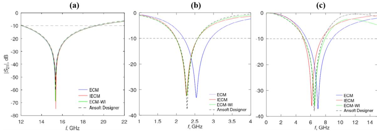
Fig. 7. Comparison between simulation results: (a) FSS 1; (b) FSS 2; (c) FSS 3.
