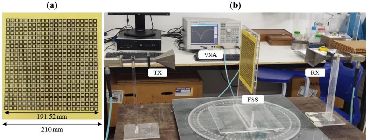
Fig. 8. Images: (a) Prototype; (b) Measurement arrangement.
