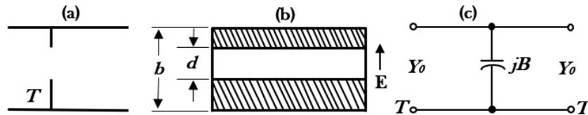
Fig. 2. Window in a rectangular waveguide: (a) side view; (b) front view; (c) equivalent circuit approximation.
