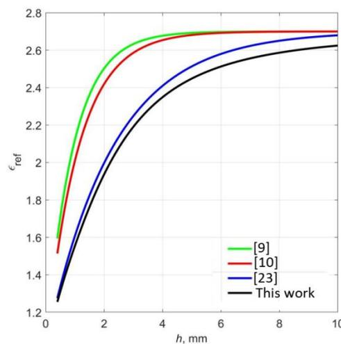
Fig. 6. Comparison between simulated results of effective electric permittivity models.
