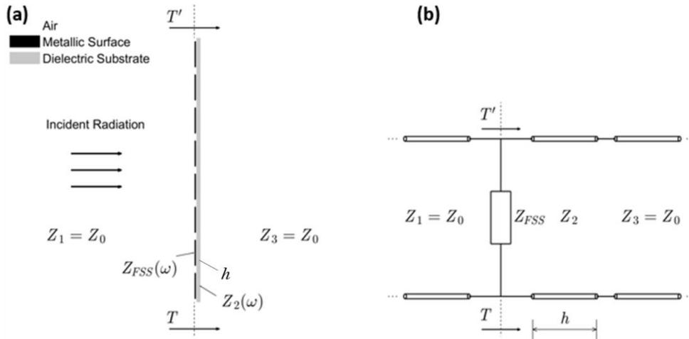
Fig. 3. FSS: (a) Representation of transmission in terms of impedances; (b) Equivalent circuit.
