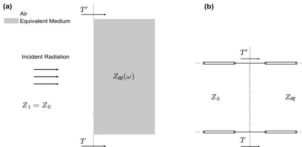
Fig. 5. FSS: (a) Representation in terms of equivalent impedance; (b) Associated equivalent circuit.
