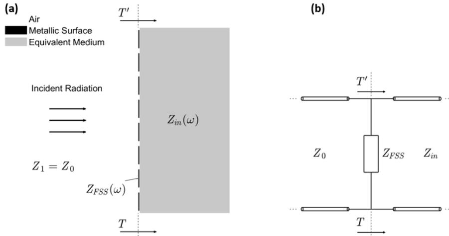
Fig. 4. FSS: (a) Illustration of the scattering problem in an FSS using the input impedance concept; (b) Equivalent circuit.
