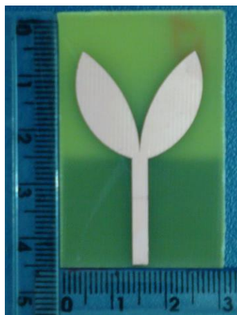
Fig. 4. Photograph of a built antenna prototype.
