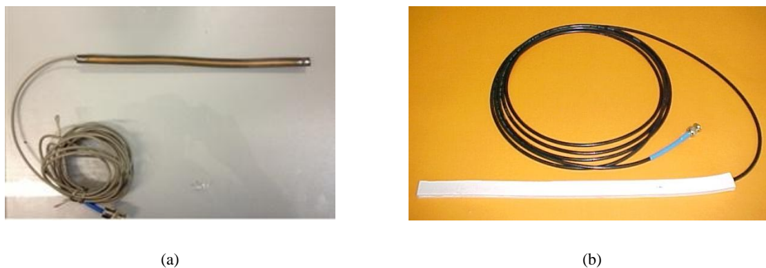
Fig.1. Duroid-based microstrip directional coupler sensor: (a) without encapsulation, (b) sensor encapsulated in silicon.
