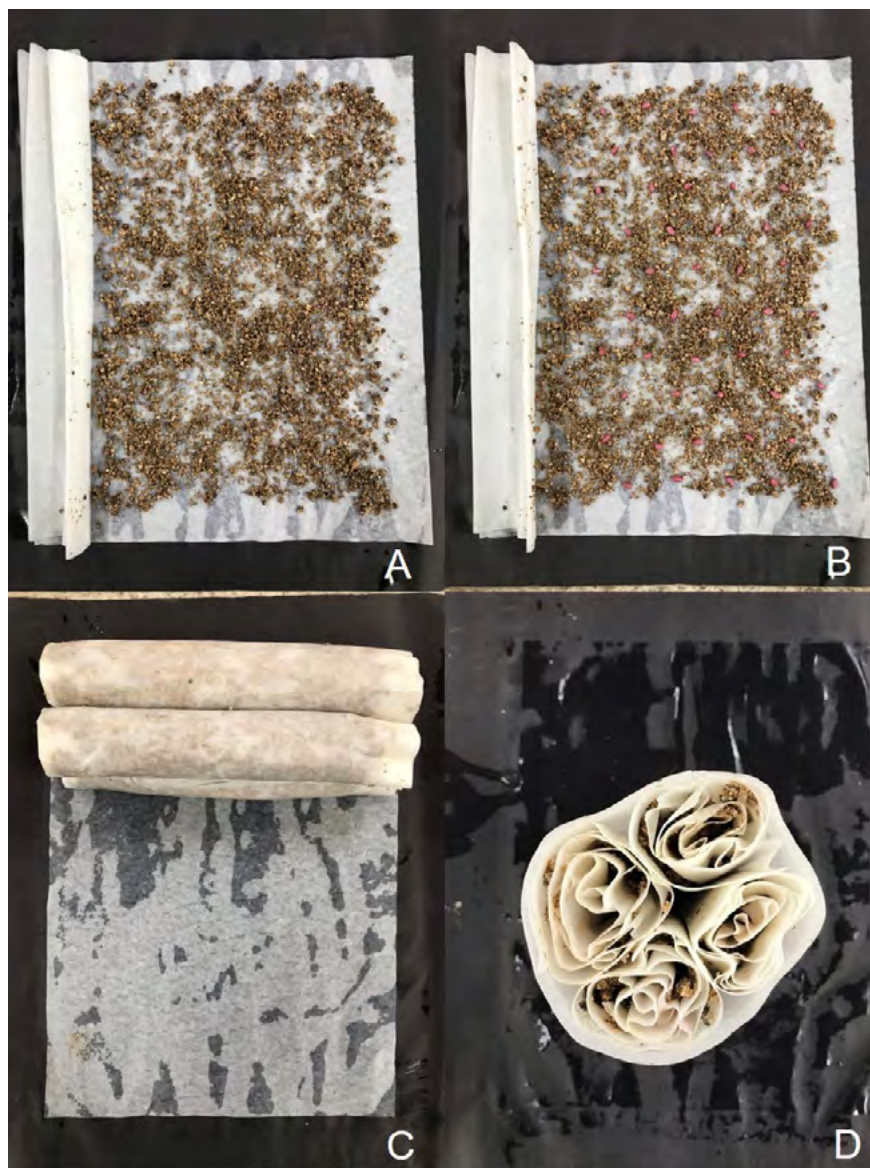
Figure 1. Methodology of setting up the alternative germination test with vermiculite, showing adequate distribution of the vermiculite (A), sowing (B), arrangement of the rolls (C), and closure of the rolls (D) (Experiment 1).
