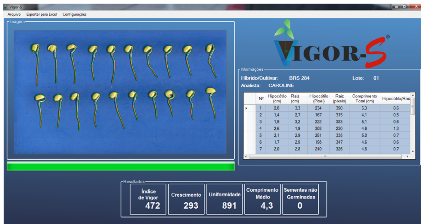
Figure 1. Analyzed images of soybean seedlings of the cultivar BRS 284, with specific demarcation of the root-hypocotyl axis, illustrating the data obtained by the Vigor-S system: vigor index, seedling uniformity and values of seedling length.
