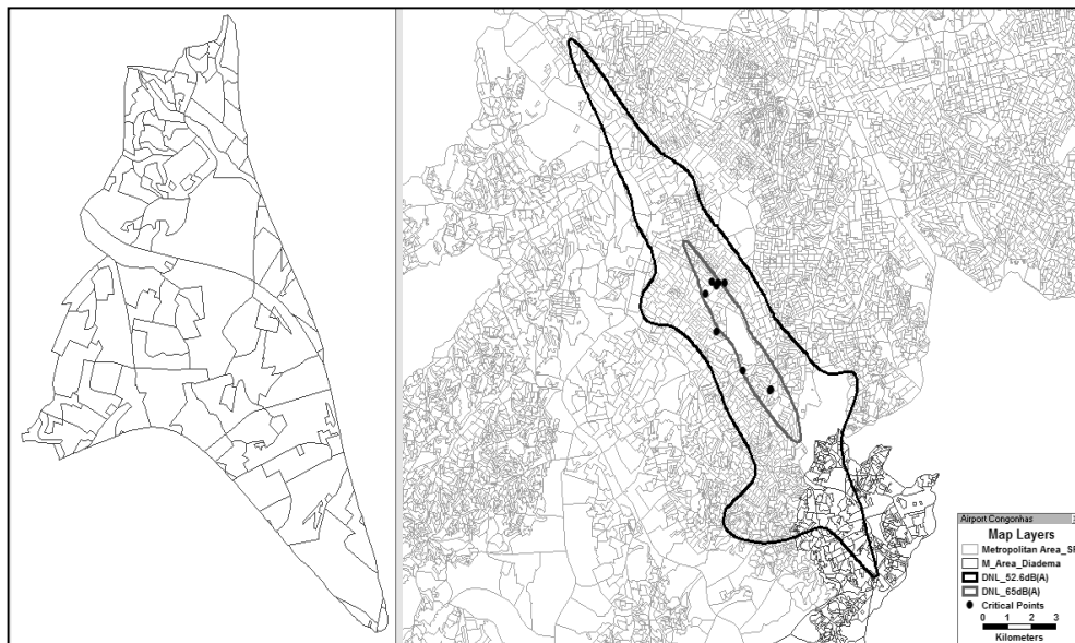
Figure 3 - Curves noise of 65 and 52.6dB(A) and critical points on the right Congonhas airport. City of Diadema inserted curve DNL 52.6dB(A) to the left 10
