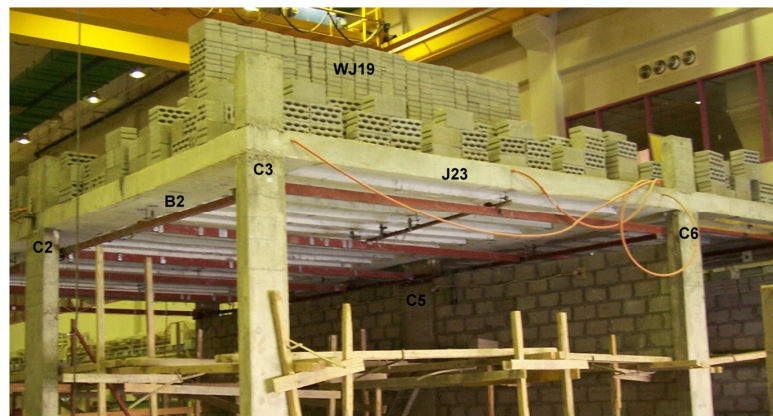
Figure 2 A photo of the tested floor showing loading and part of the geometry
