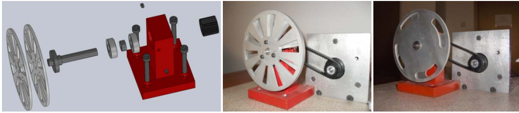
Figure 9 Chopper module: blueprint (a); assembly of the wheels with linear (b) and with circular outward (c) edges.
