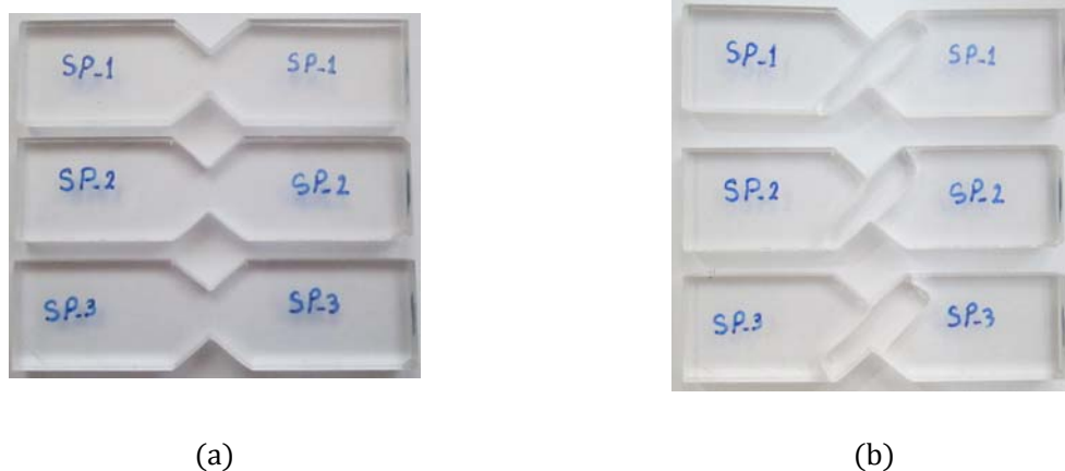
Figure 11: PMMA test specimen (a) and (b) indicate the before and after test, respectively.
