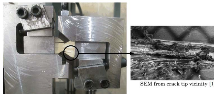
Figure 10: SEM photo from crack tip vicinity of wood specimen
