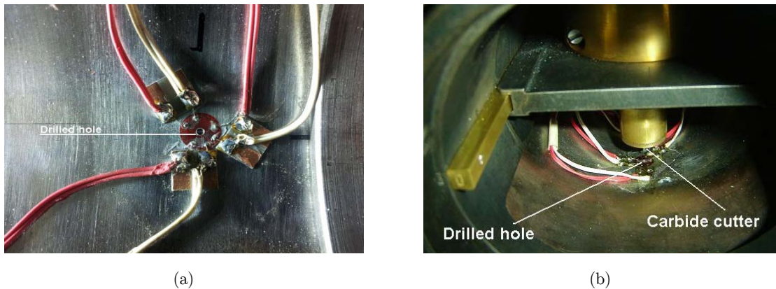
Figure 9: a) Rosette with the drilled hole; b) Drilling a hole in the inside wall Mock-up.
