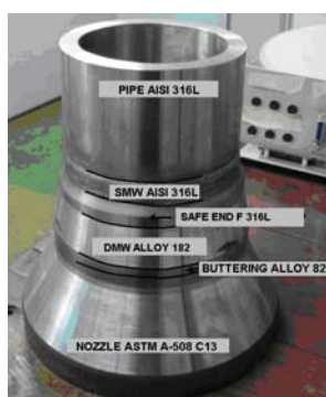
Figure 5: Mock-up that simulates Angra 1 NPP nozzle.
