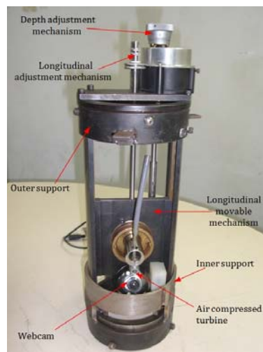
Figure 1: Developed equipment to assist measuring residual stresses inside wall pipes.
